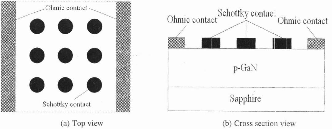
Figure 1: (a) Top view, and (b) cross section view of ohmic and Schottky contacts of a typical sample
