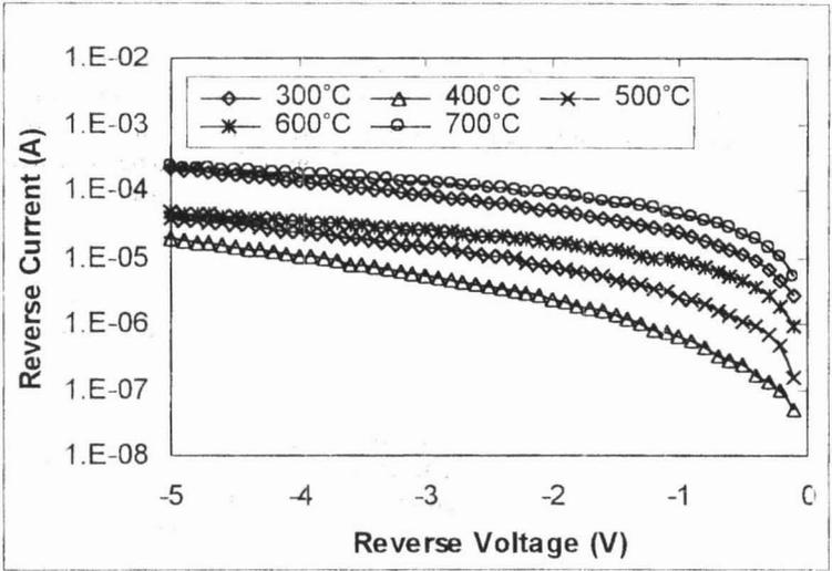
Figure 3: The reverse I-V characteristics of Pd/p-GaN annealed at various temperatures for 35 minutes
