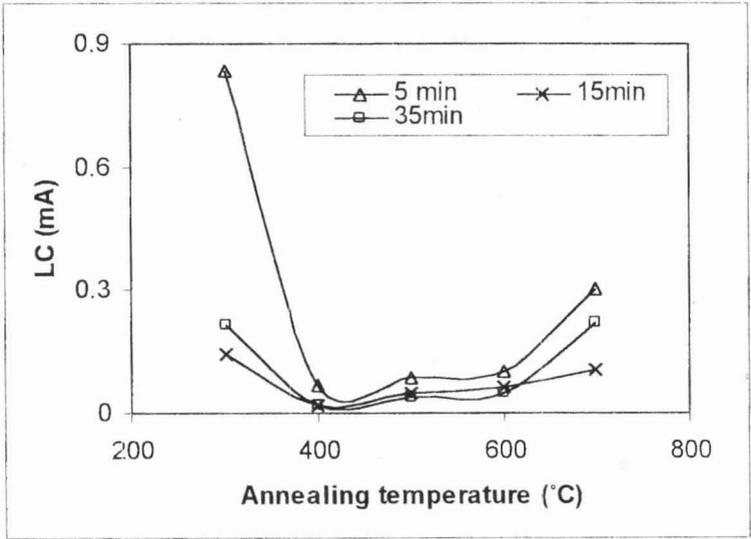
Figure 4: The changes of leakage current versus annealing temperatures for various annealing times
