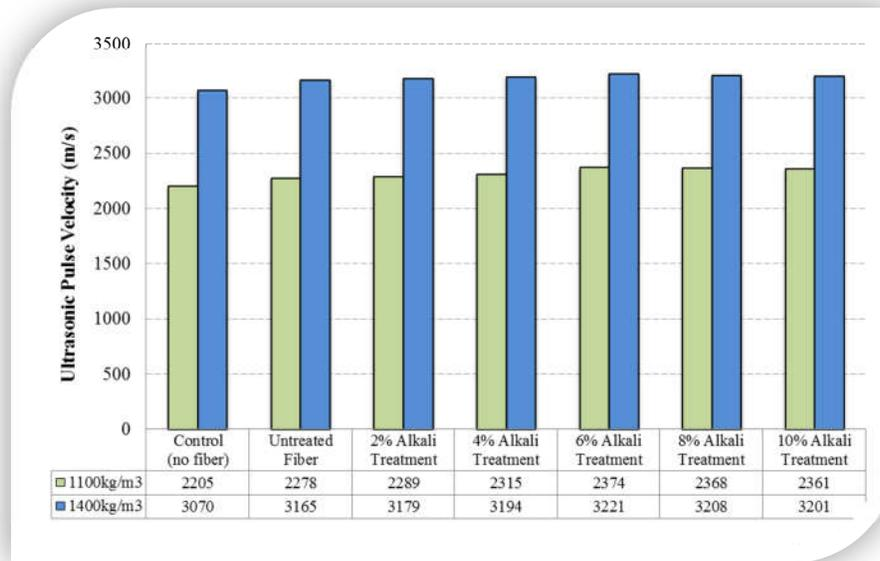
Figure 5: Influence of alkali treatment of coir fiber on ultrasonic pulse velocity of foamed concrete
