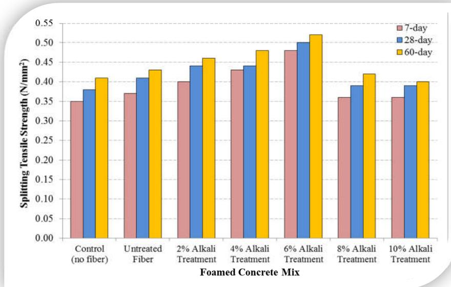
Figure 8: Influence of alkali treatment of coir fiber on splitting tensile strength for 1100kg/m<sup>3</sup> density
