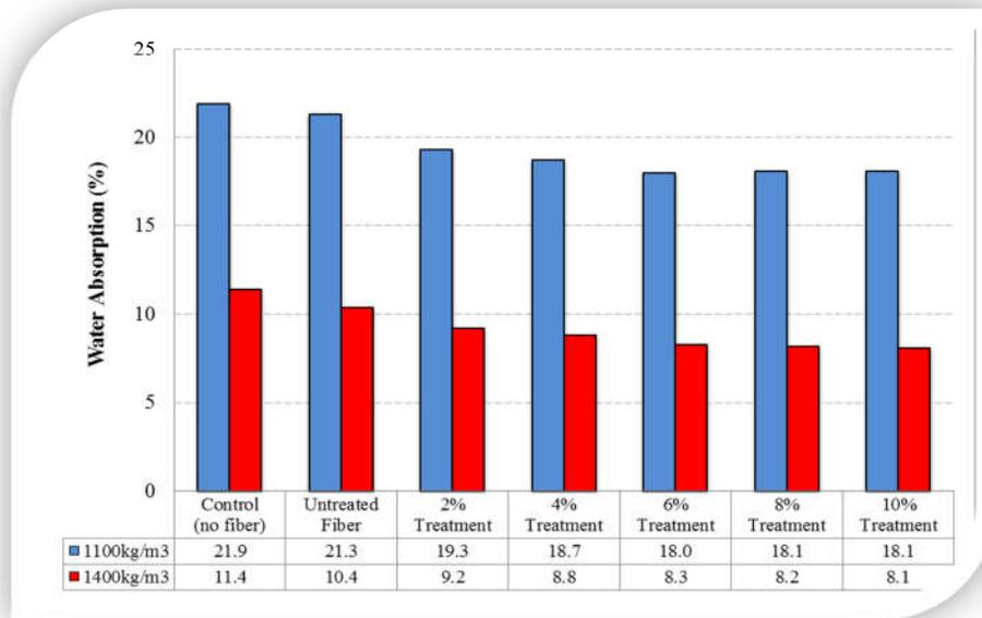
Figure 3: Influence of alkali treatment of coir fiber on moisture absorption capacity of foamed concrete
