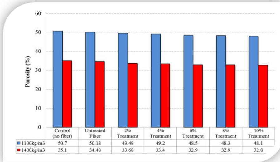
Figure 4: Influence of alkali treatment of coir fiber on porosity of foamed concrete
