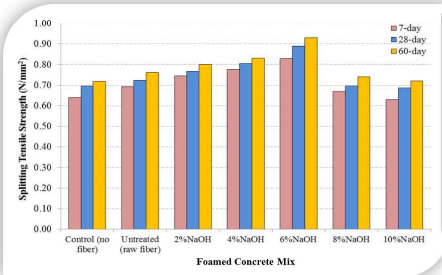
Figure 9: Influence of alkali treatment of coir fiber on splitting tensile strength for 1400kg/m<sup>3</sup> density
