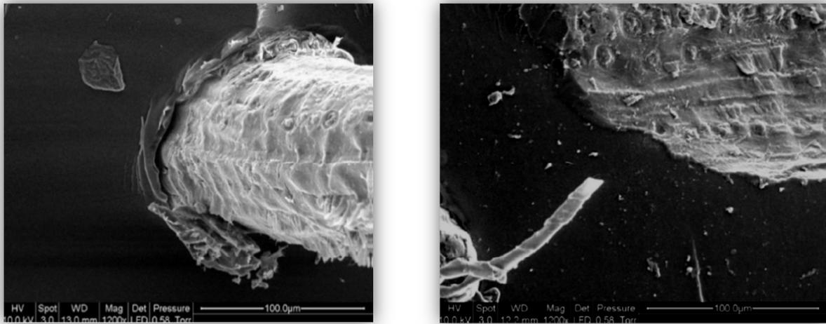
Figure 10: SEM results of coir fiber-cement interface: untreated (left) & treated (right)
