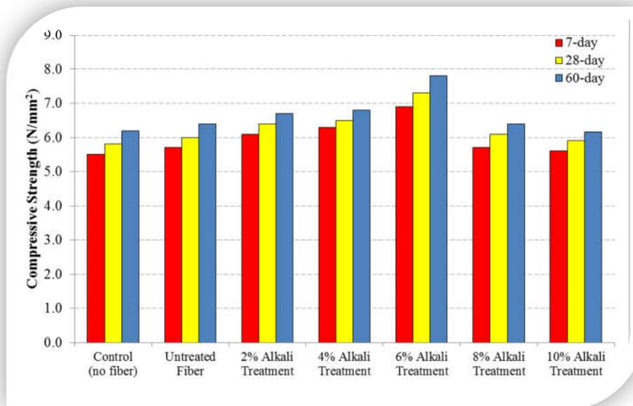
Figure 7: Influence of alkali treatment of coir fiber on compressive strength for 1400kg/m<sup>3</sup> density
