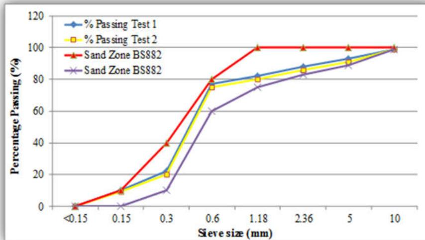
Figure 1: Sieve analysis grading result
