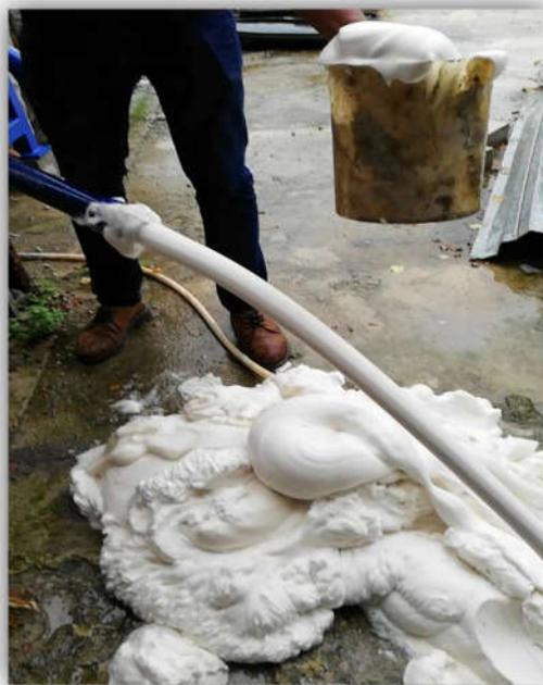
Figure 2: Production of stable foam via Portaform TM-2 machine
