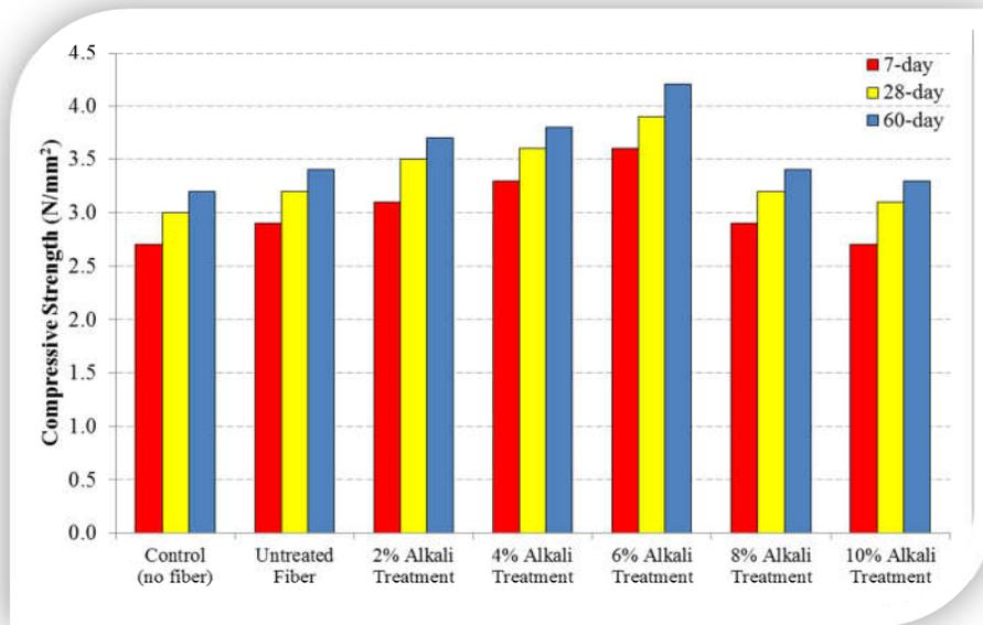
Figure 6: Influence of alkali treatment of coir fiber on compressive strength for 1100kg/m<sup>3</sup> density
