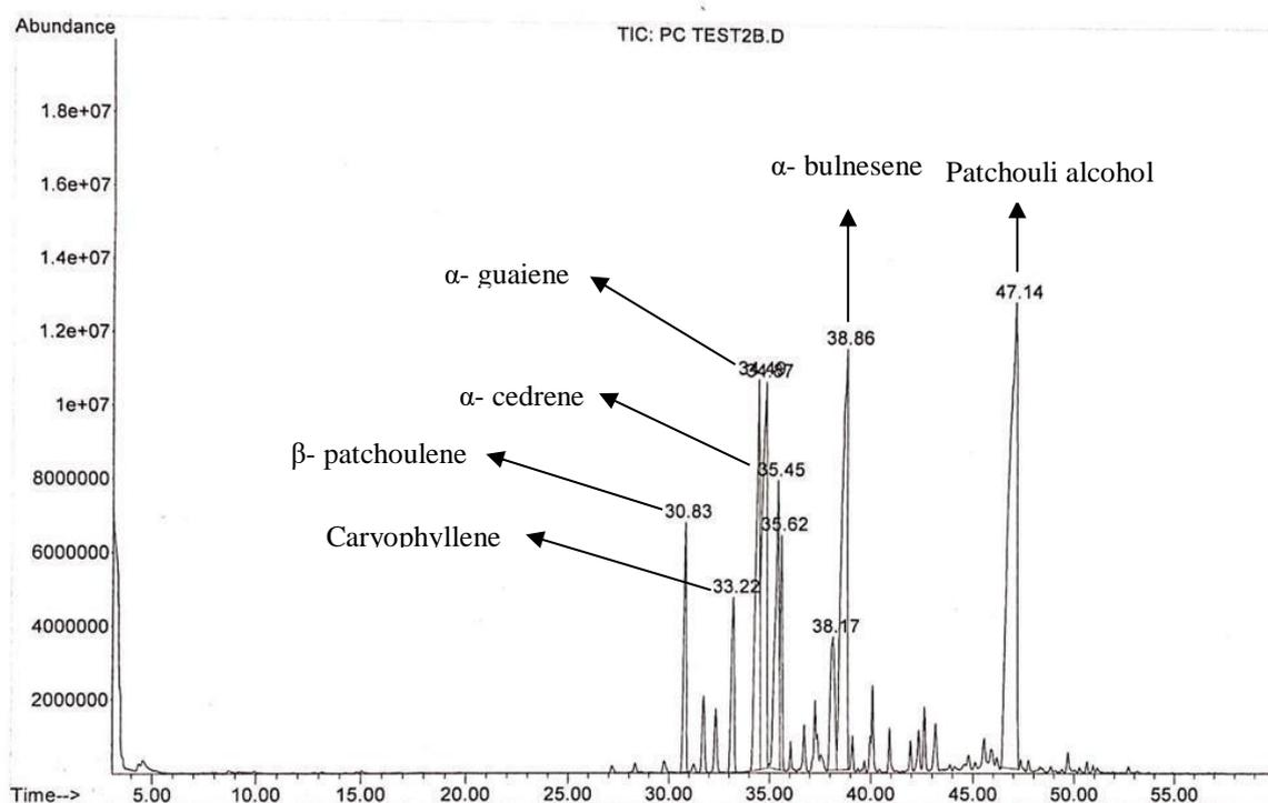
Figure 7: The chromatogram of *ex vitro* *P.cablin* using GC-MS
