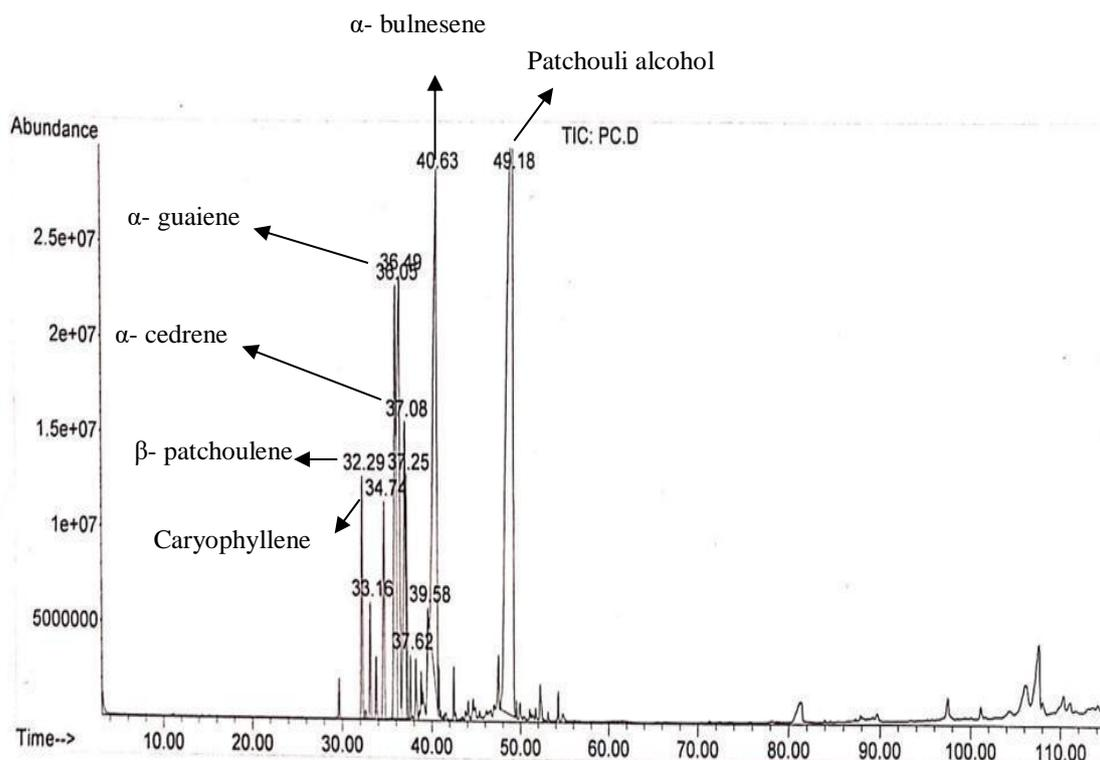
Figure 6: The chromatogram of *in vitro* *P.cablin* using GC-MS
