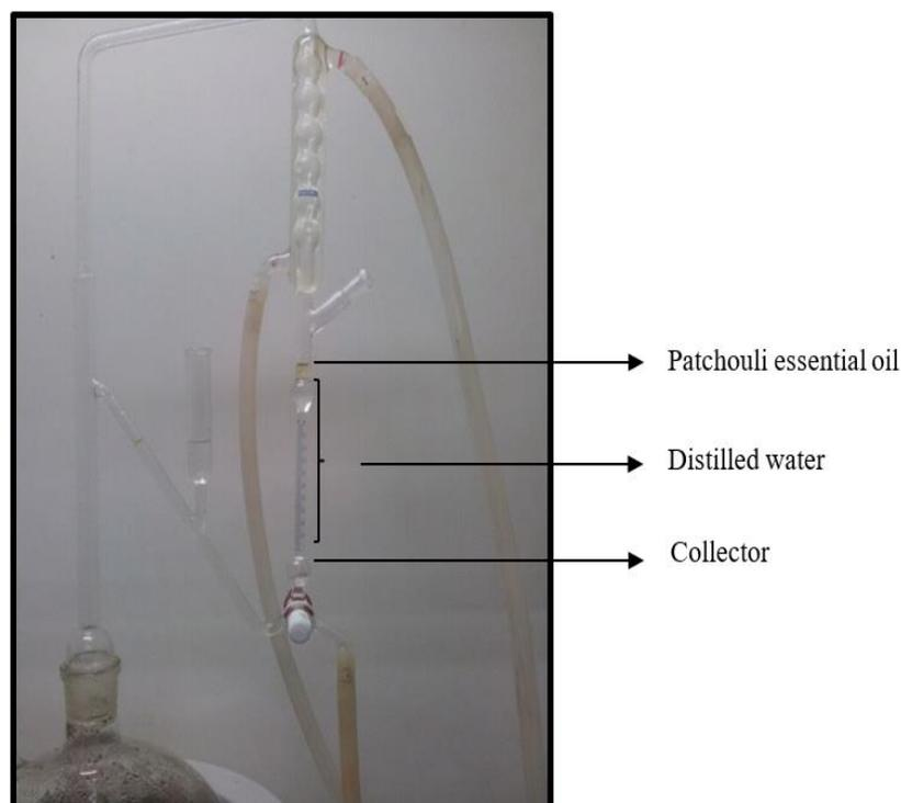
Figure 4: The Oil And Distillated Water Were Dispensed And Collected Through The Collector Tube
