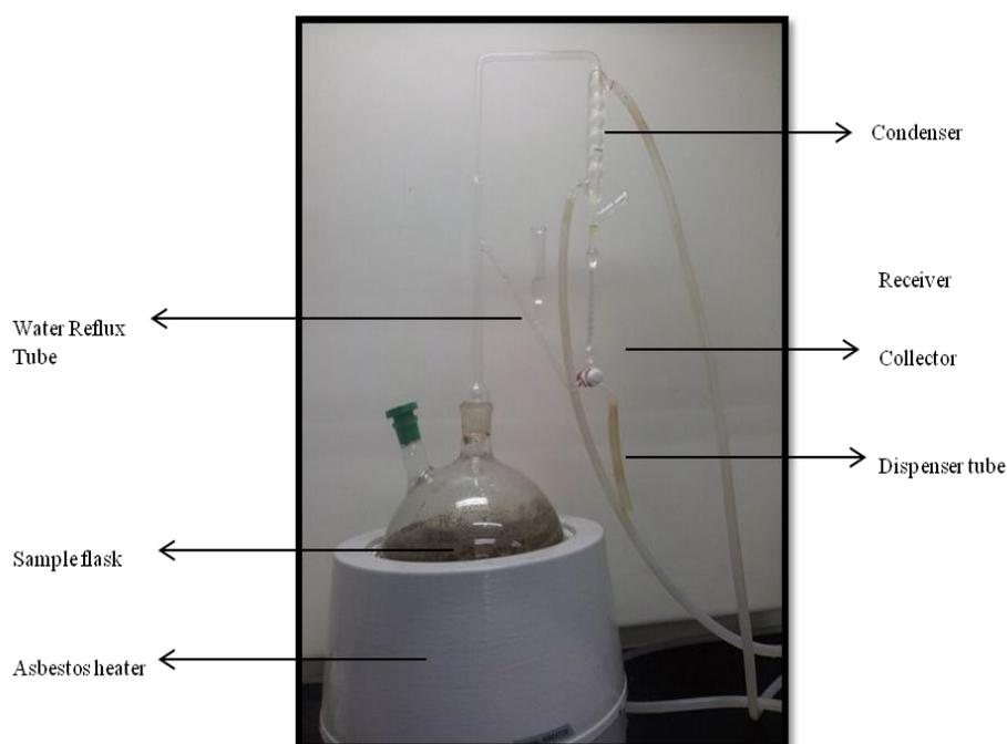
Figure 3: The Clevenger Apparatus Set for Hydrodistillation Process of Patchouli Essential Oil
