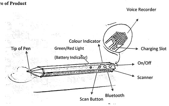
Figure 1.0 Physical View of the Miracle Pen
