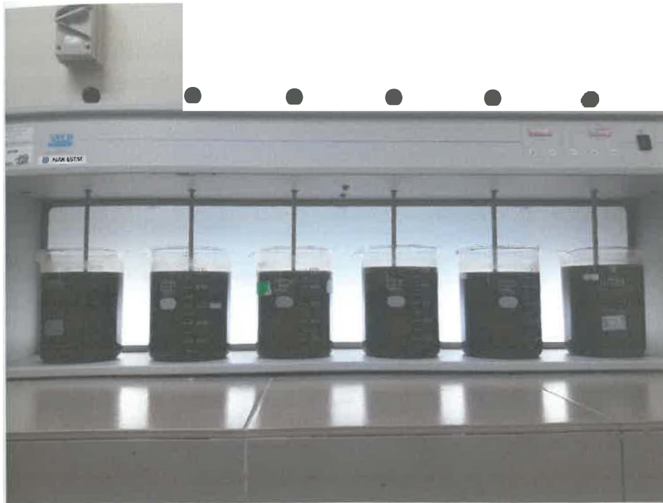
Fig. 2 : Six (6) jar test were filled with 1000mL of POME
