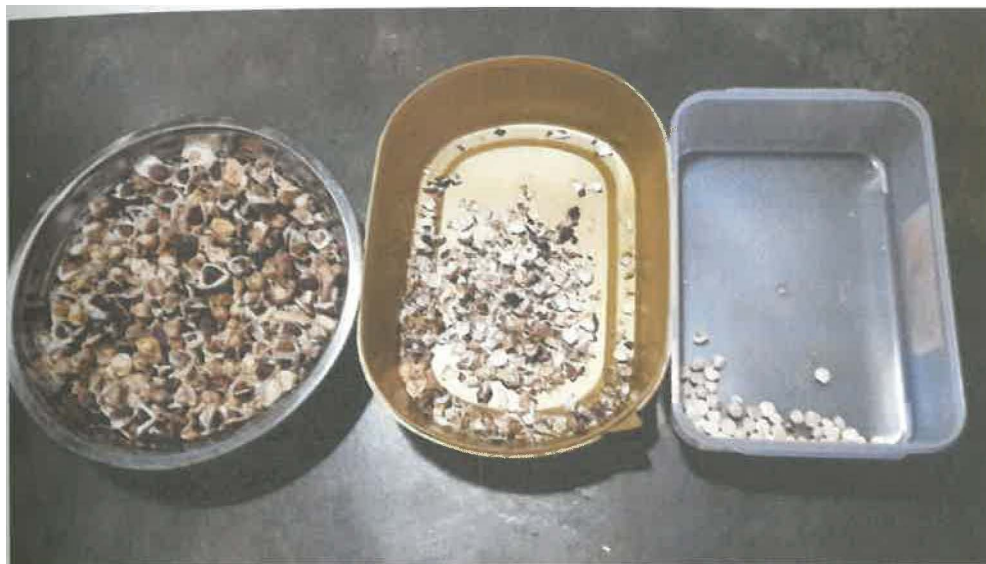
Fig. 1 : Moringa oleifera seeds for POME pretreatment.
