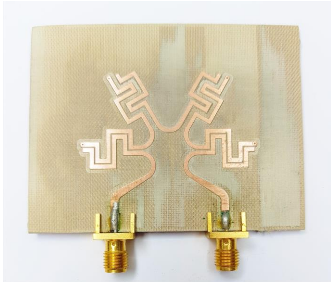
Fig. 12. Photograph of the 3 rd order meandered lines bandpass filter.
