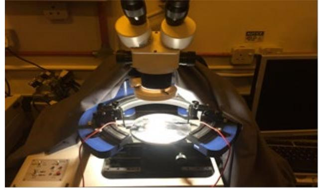
Fig. 8. Measurement setup to calculate conductivity of electro-textile sample based on I.V curve
