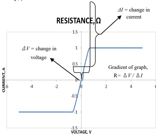
Fig. 7. Extracted resistance value from the I-V probe measurement tool
