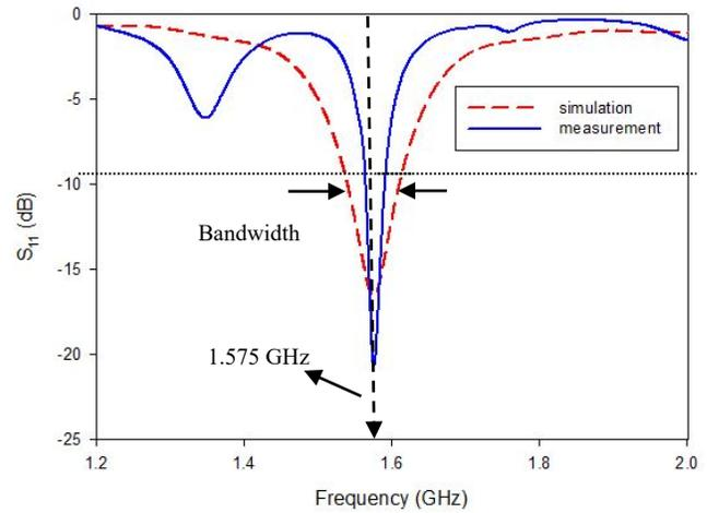
Fig.11. Comparison between simulation and experimental data obtained for the return loss of the electro-textile antenna
