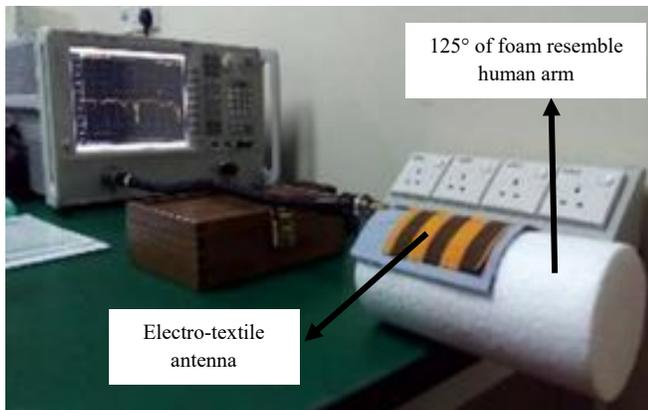
Fig. 16. Electro-textile antenna in bent condition on 125° foam
