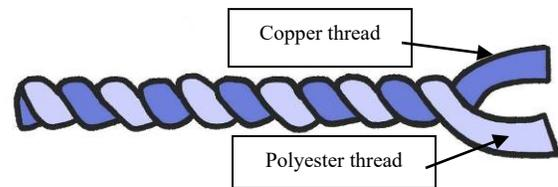
Fig. 3. Twisting technique used for copper-covered yarn construction
