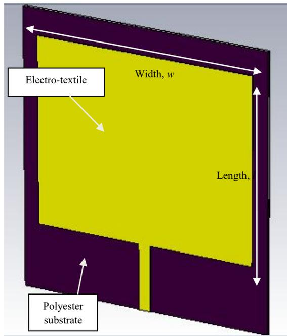
Fig. 9. Electro-textile antenna designed in CST solver
