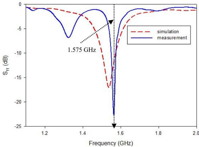
Fig.15. Comparison of S<sub>11</sub> between simulation and experimental data obtained for bent condition
