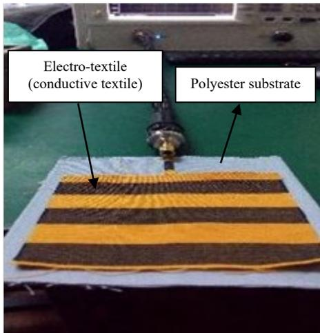
Fig. 10. Electro-textile antenna on polyester fabric
