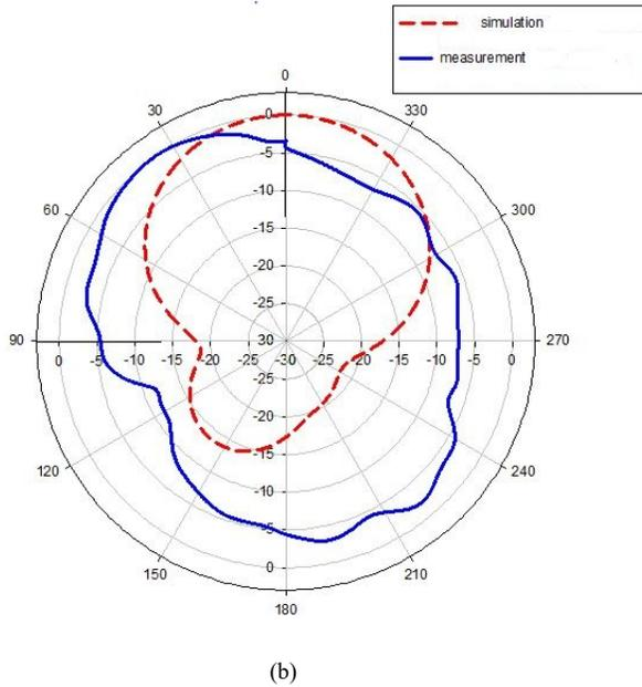
Fig. 17. (a) Simulated and measured radiation patterns of the electro-textile antenna on bent condition for E-plane (yz-plane) (b) Simulated and measured radiation patterns of the electro-textile antenna on bent condition for H-plane (xz-plane)
