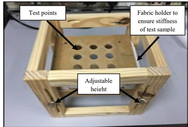
Fig. 6. Measurement tool (jig) for textile parametric measurement
