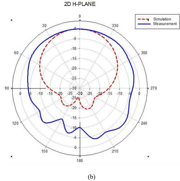
Fig. 13. a) Simulated and measured radiation patterns of the electro-textile antenna at 1.575GHz for E-plane ( $yz$ -plane). b) Simulated and measured radiation patterns of the electro-textile antenna at 1.575GHz for H-plane ( $xz$ -plane)
