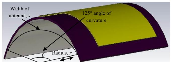
Fig. 14. Electro-textile antenna in bent condition at  $125^\circ$  angle of curvature in CST simulation
