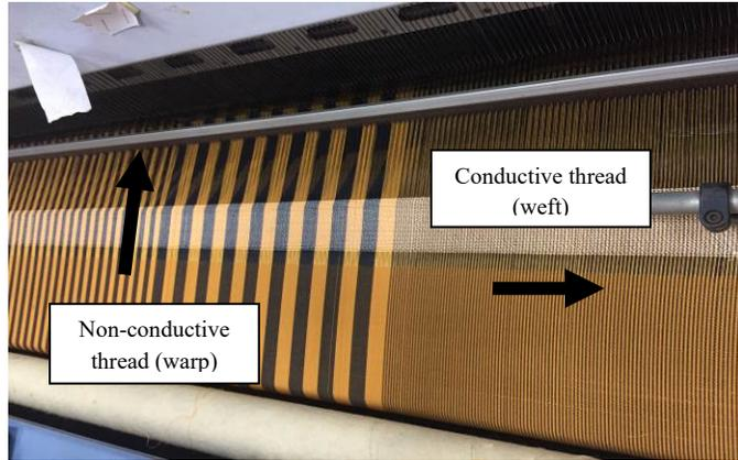
Fig. 5. Warp and weft of electro-textile fabric
