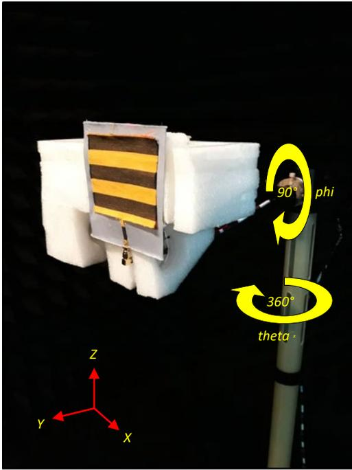
Fig. 12. Experimental setup of electro-textile antenna in an anechoic chamber for far-field radiation patterns
