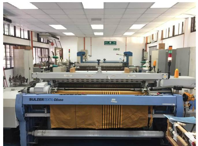
Fig. 4. SULZER TEXTIL G6300 rapier weaving machine
