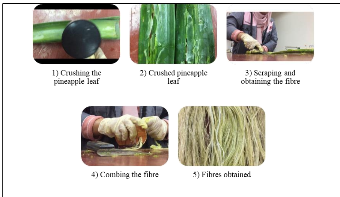
Figure 2. Extraction process of pineapple leaf fibres
