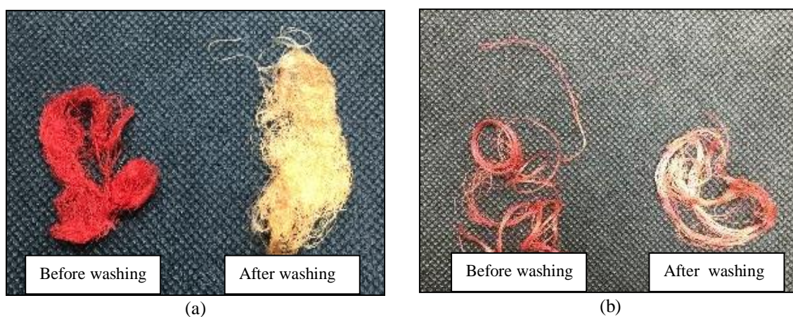
Figure 6. Colour change of pineapple leaf fibres for a) Infrared dyeing machine and b) Exhaustion dyeing machine
