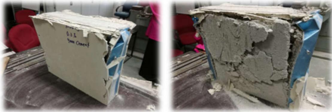
Figure 5: Failure mode of plain foamcrete of 1000 kg/m<sup>3</sup> density core and 9mm fiber cement board outer skins
