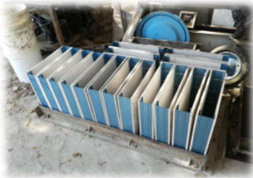
Figure 1: Preparation of outer skins of SIPs
