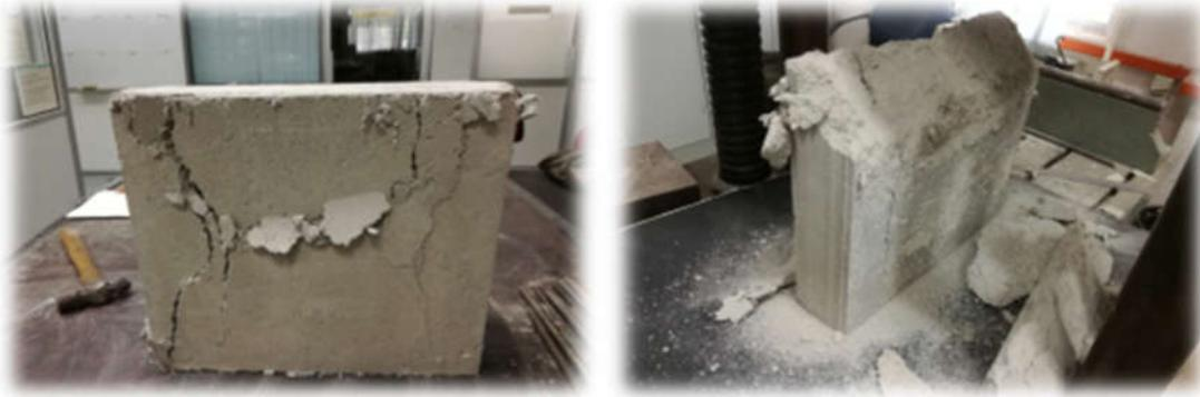
Figure 3: Failure mode of plain foamcrete of 1000 kg/m<sup>3</sup> density
