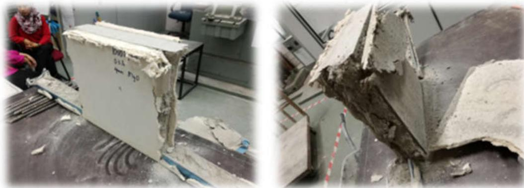
Figure 6: Failure mode of plain foamcrete of 1000 kg/m<sup>3</sup> density core and 9mm MgO board outer skins
