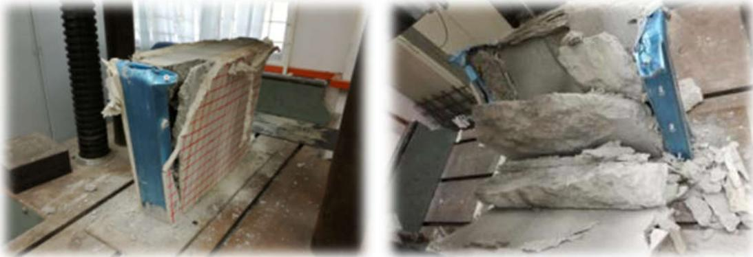
Figure 4: Failure mode of plain foamcrete of 1000 kg/m<sup>3</sup> density core and 8mm fiber cement board outer skins
