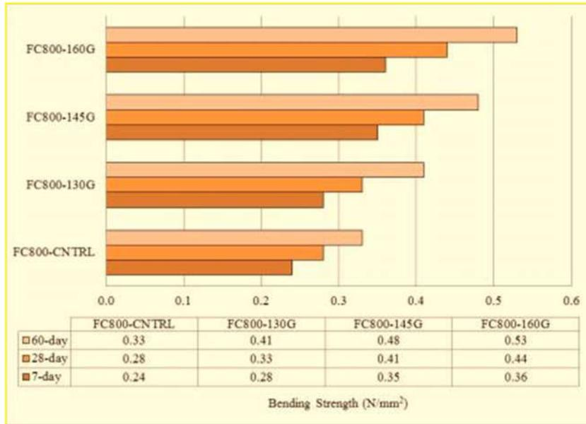
Figure 6: Influence of different types of textile carbon grid laminates on bending strength of 800kg/m<sup>3</sup> density
