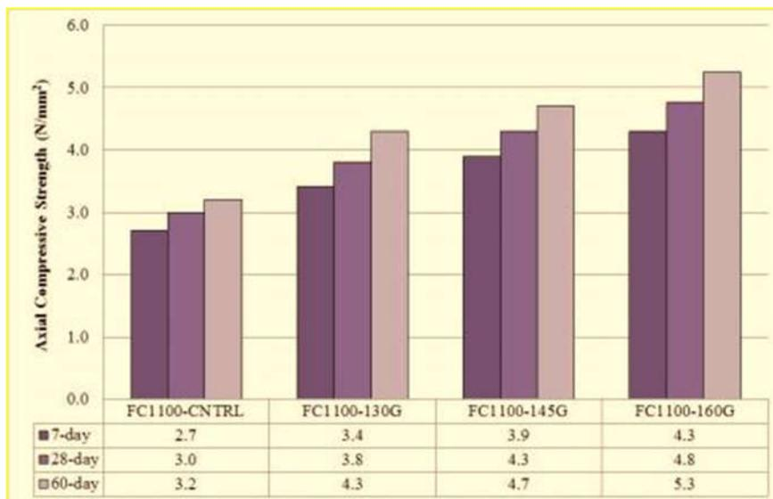
Figure 4: Influence of different types of textile carbon grid laminates on compressive strength of 1100kg/m<sup>3</sup> density
