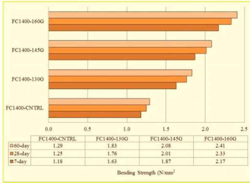
Figure 8: Influence of different types of textile carbon grid laminates on bending strength of 1400kg/m<sup>3</sup> density
