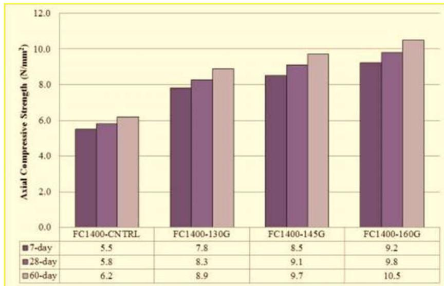
Figure 5: Influence of different types of textile carbon grid laminates on compressive strength of 1400kg/m<sup>3</sup> density
