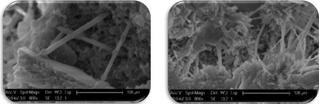
Figure 10: SEM micrographs of fracture surface of cement matrix reinforced with textile carbon grid laminates
