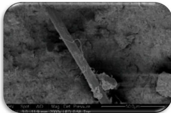
Figure 11: SEM micrographs of pull-out of textile carbon grid laminates from cement matrix
