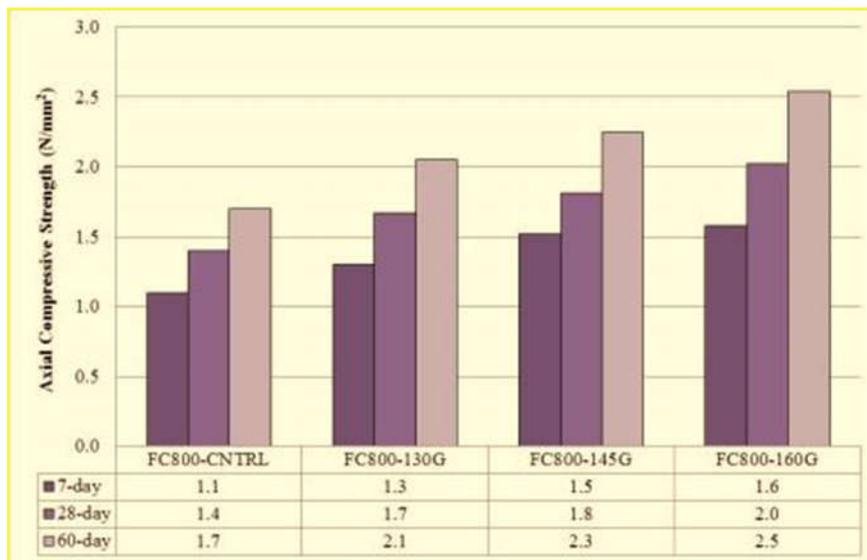
Figure 3: Influence of different types of textile carbon grid laminates on compressive strength of 800kg/m<sup>3</sup> density
