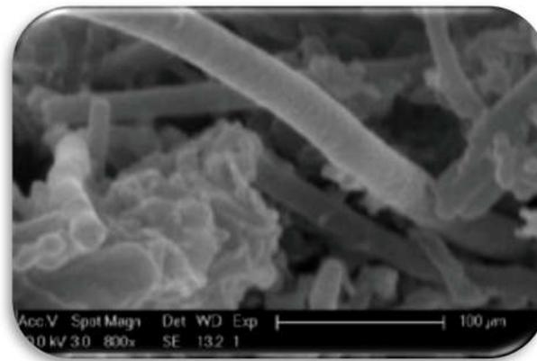
Figure 9: Morphology of textile carbon grid laminates in cement matrix
