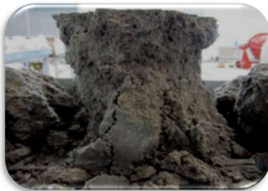
Figure 16: Plain (control) foamed mortar sample after failure under axial compression
