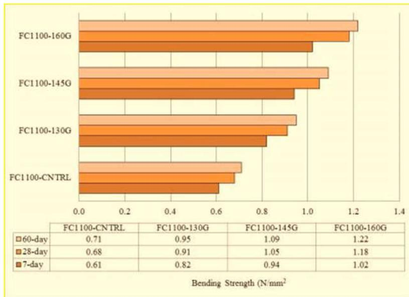
Figure 7: Influence of different types of textile carbon grid laminates on bending strength of 1100kg/m<sup>3</sup> density
