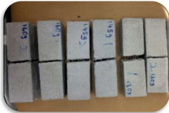
Figure 19: Textile carbon grid laminates reinforced foamed concrete sample after failure under three-point bending strength
