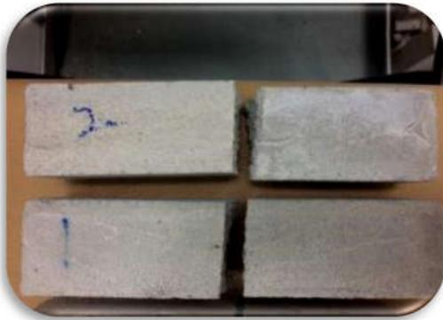
Figure 18: Plain (control) foamed mortar sample after failure under three-point bending strength
