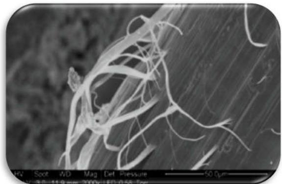
Figure 12: SEM micrographs of textile carbon grid laminates surface in a failed specimen under flexural load
