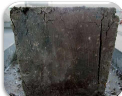
Figure 17: Textile carbon grid laminates reinforced foamed mortar sample after failure under axial compression
