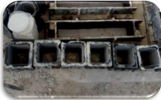
Figure 1: Textile carbon grid laminates was cut into different sizes to fit into the moulds
