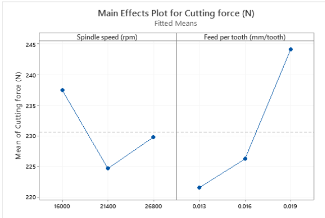
Figure 6: Main effects in terms of mean of cutting force (N) values for half-immersion down-milling.
