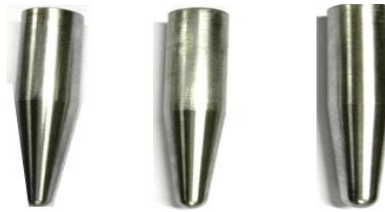
Figure 5: Forming tools with \Phi 8 , \Phi 10 and \Phi 12 diameter spherical end.
