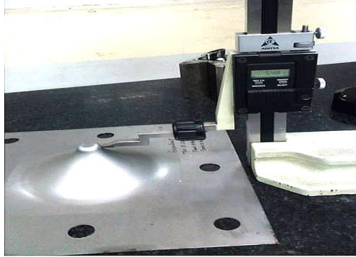
Figure 13: Depth measurement method using Vernier Height Gauge.
