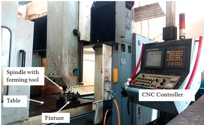
Figure 6: Experimental setup for single point incremental forming.
