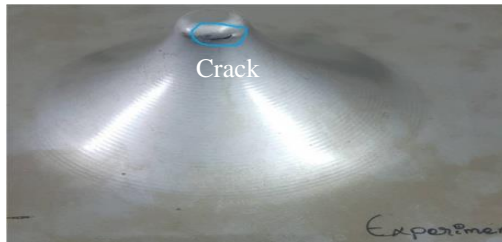
Figure 14: Magnified view of the crack formed in experiment 1.
