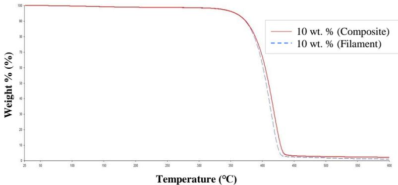
Figure 6: Thermal degradation of PLA-OPEFBF composites and filaments.
