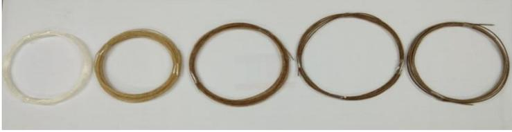
Figure 3: Successfully extruded filaments (Code: 0, 10, 20, 30, and 40).
