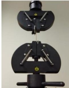
Figure 2: Tensile testing setup of PLA-OPEFBF filament.
