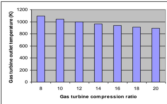
Figure 4: Effect of the compression ratio of the gas turbine on gas turbine outlet temperature.
