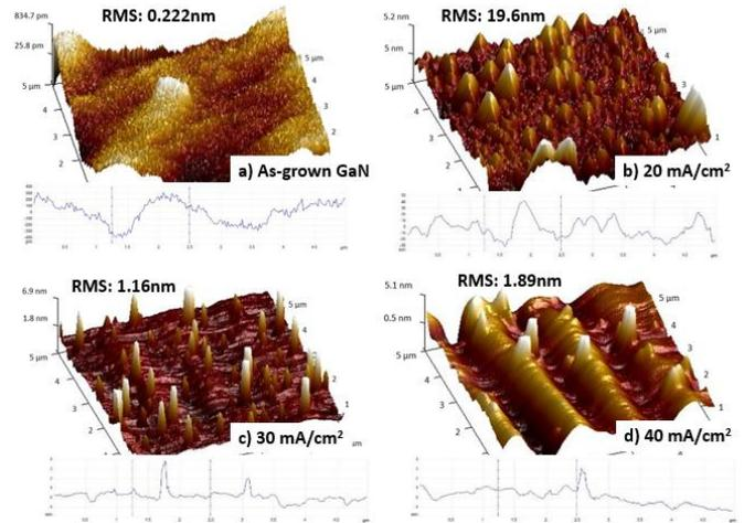
Fig. 3. 3D images and cross section line scan of a) as-grown GaN and all porous GaN samples fabricated with current density of b) 20 mA/cm<sup>2</sup>, c) 30mA/cm<sup>2</sup> and d) 40mA/cm<sup>2</sup>.
