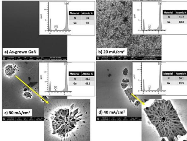
Fig. 2. SEM images and EDX of a) as-grown GaN and all PGaN samples fabricated with current density of b) 20 mA/cm<sup>2</sup>, c) 30mA/cm<sup>2</sup> and d) 40mA/cm<sup>2</sup>.
