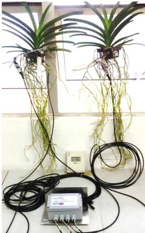
Fig. 3. The dendrometers secured to the vandaceous root structure, along with temperature and humidity sensors.
