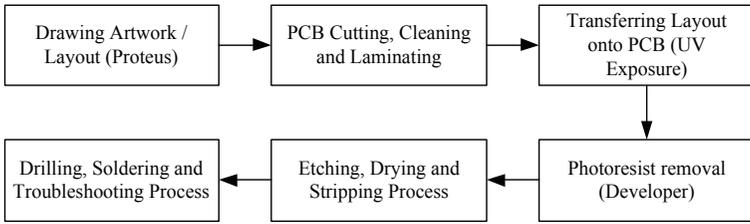
**Figure 3: PCB fabrication process**
