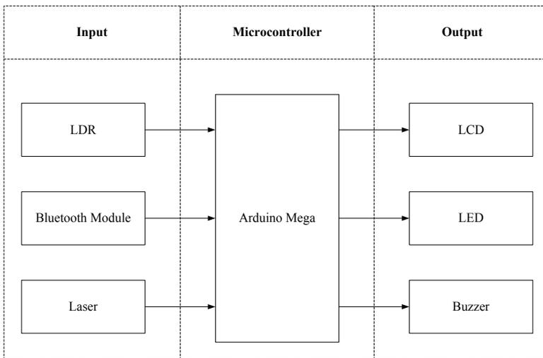
**Figure 2: Block diagram of the prototype**
