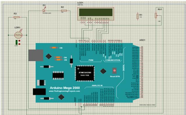
**Figure 4: Schematic diagram of the prototype**
