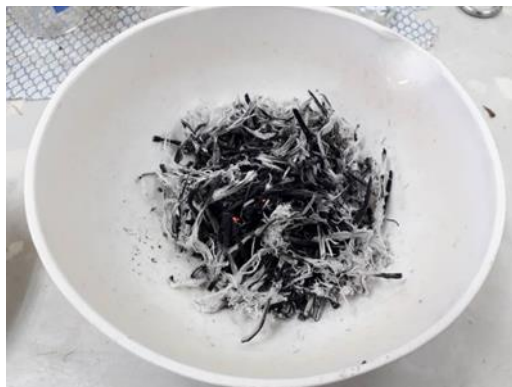
Figure 1 The EFB ashes after burned in the furnace at 550°C
