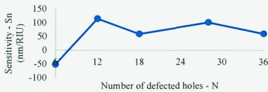
Fig. 15(a): RI sensitivity, Q factor and normalized transmittance of PhC microcavity ( r_1 = 0.45a ) when N=6, 12, 18, 28, and 36 .
