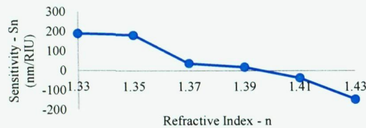
Fig.13(c): RI sensitivity of PhC microcavity ( r_1=0.45a , N=6 ) when the RI ranged from 1.33 to 1.43.
