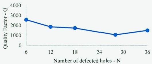
Fig. 15(b): Q factor of PhC microcavity ( r_1 = 0.45a ) when N=6, 12, 18, 28, and 36 .
