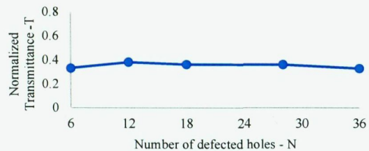
Fig. 15(c): Normalized transmittance of PhC microcavity ( r_1 = 0.45a ) when N=6, 12, 18, 28, and 36 .
