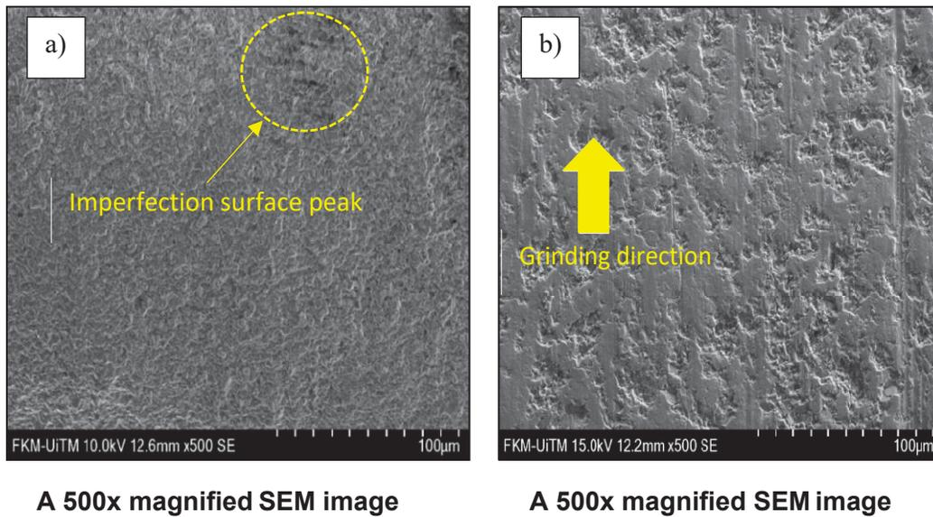
**Figure 6: SEM Image a) Before Grinding b) After Grinding**
