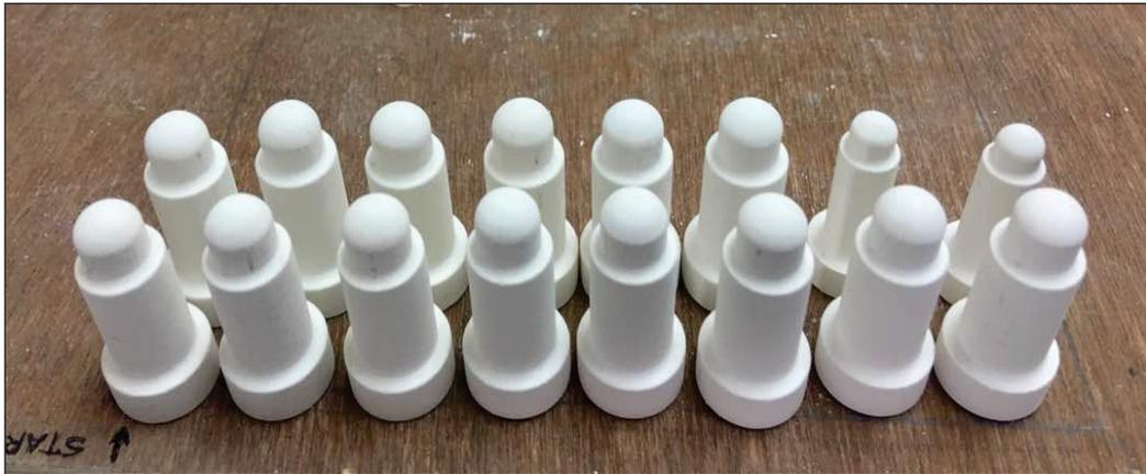
**Figure 1: Alumina Sintered Guide Pin Manufactured by RSAT Sdn. Bhd
