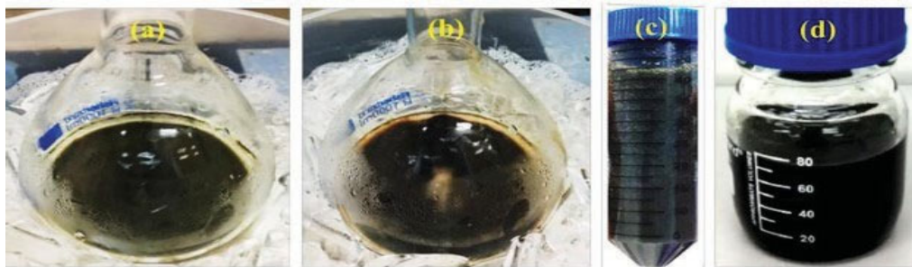
Figure 2: Mixture of GO Solution using Modifies Hummer's Method After (a) Added 50 ml of DI and (b) Added 100 ml of DI Water for the Three Hours of Stirring Under an Ice Bath Setup. GO Solution Produced After Sited-Down Overnight and Discard the Excess Water with Reaction Stirring Time of (c) One Hours 30 Minutes and (d) Three Hours
