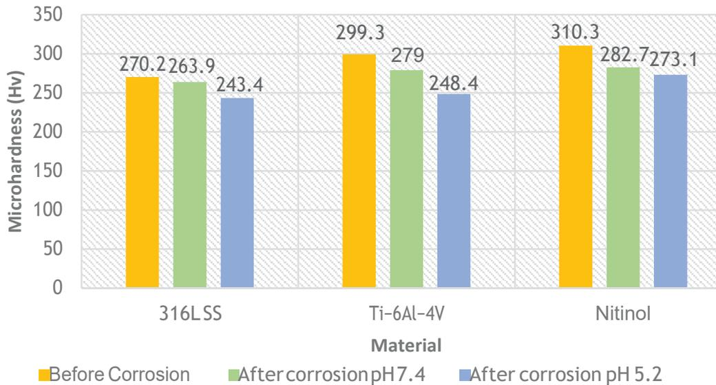
Figure 9: The Bar Chart of Microhardness under the Condition Before and After Corrosion
