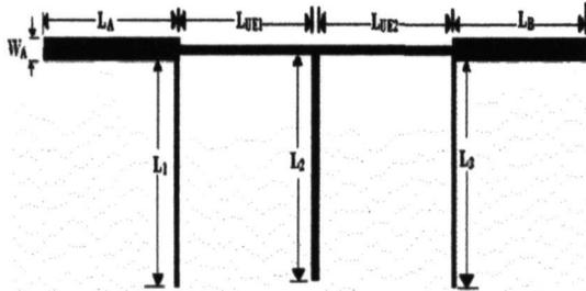
Figure 3: dimension of the proposed filter.
