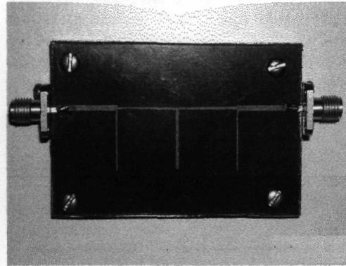
Figure 7: the realization of the microstrip bandstop filter.
