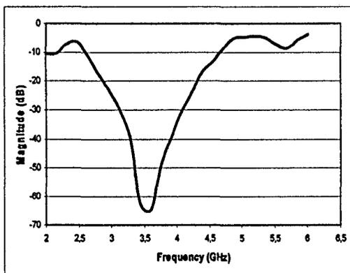
Figure 8: Insertion loss measured using scalar network analyzer
