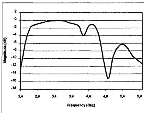
Figure 9: Return loss measured using scalar network analyzer
