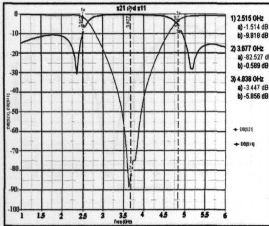
Fig 5: Simulated insertion loss and return lost of second filter design.
