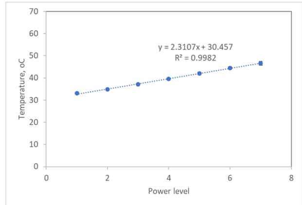
Fig. 1 Calibration curve for tray dryer
