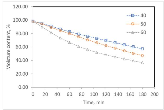
Fig. 3 Drying curve of mango in oven dryer
