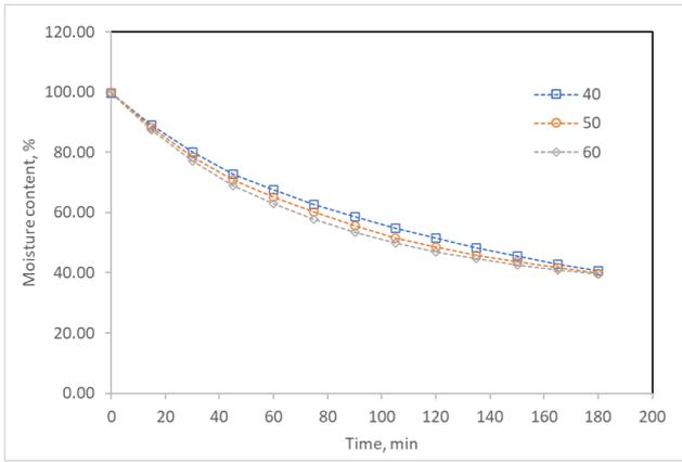
Fig. 2 Drying curve of mango in tray dryer
