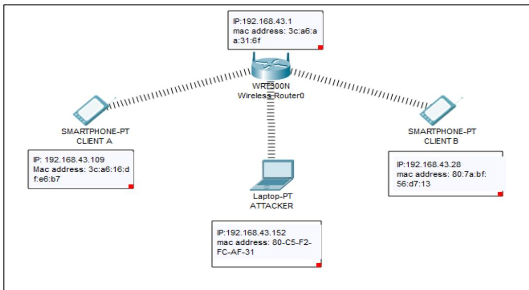
Figure 1 Testbed architecture
