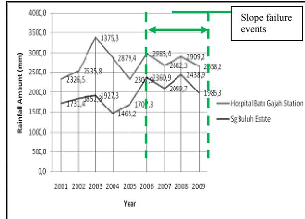
Figure 5: Yearly rainfall amount and slope failure events
