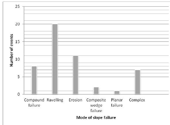
Figure 1: Mode of failure on forty nine (49) sedimentary slope
