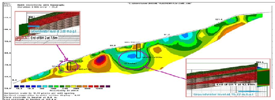
Figure 7: Comparison between Soil Profiles and Resistivity Values at Location 2 Slim River
