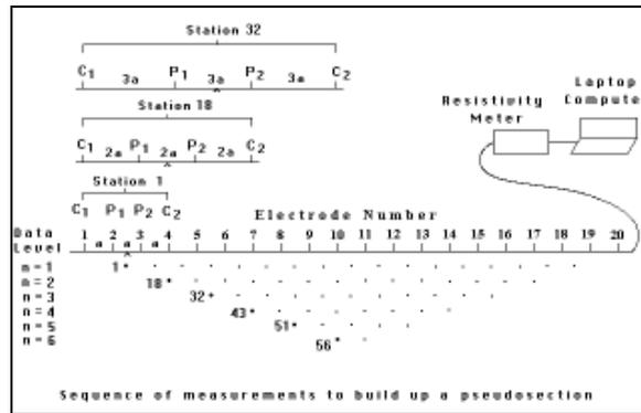
Figure 3: Two-dimensional electrical resistivity survey.
