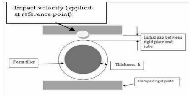
Figure 1: Finite element modeling of lateral collapse of foam filled tube
