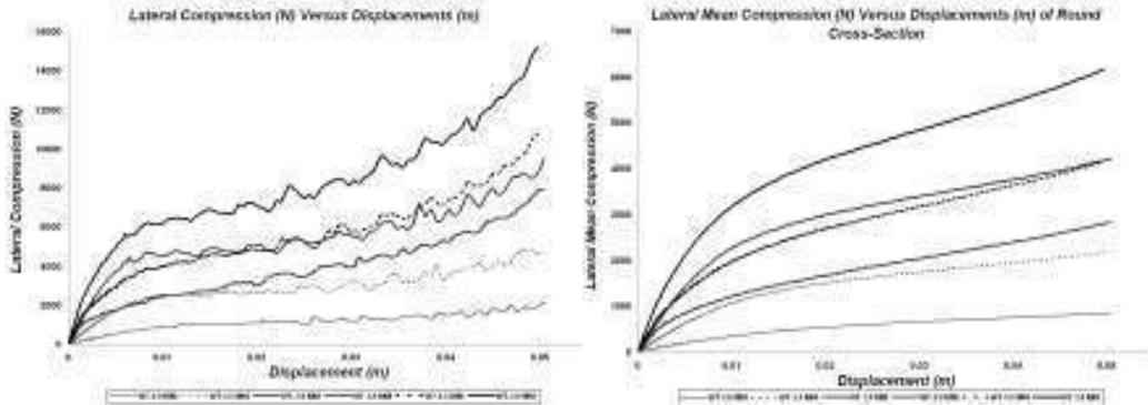
Figure 3: Quasi-static lateral load (N) versus displacement (m) type of circular tube profile (Black – with foam; Red without foam) [Wall-Thickness = 1.0, 1.5, and 2.0 mm]
