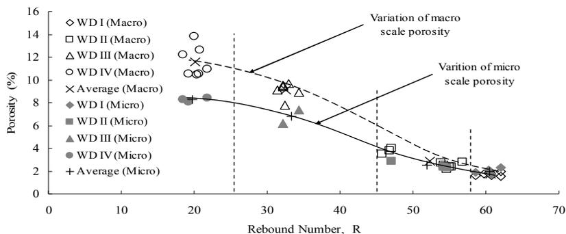
Figure 5: Variation of micro and macro scale porosity depending on the degree of weathering
