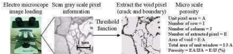
Figure 3: Analytical image processing from petrographic thin section slide
