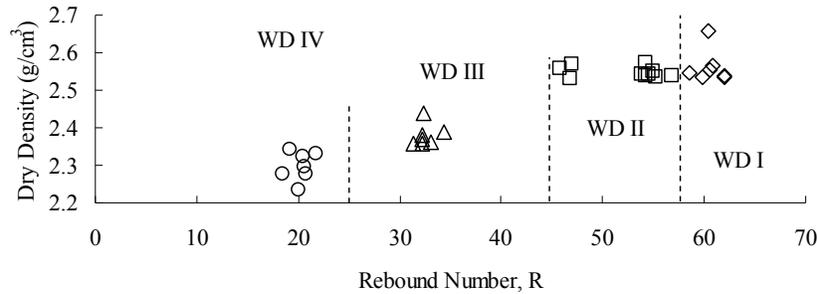
Figure 2: Rebound number and dry density of collected granite samples. Note: WD denotes weathering degree.
