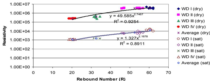
Figure 8: Electrical resistivity depending on weathering degree
