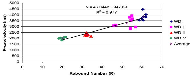
Figure 7: P-wave velocity depending on weathering degree
