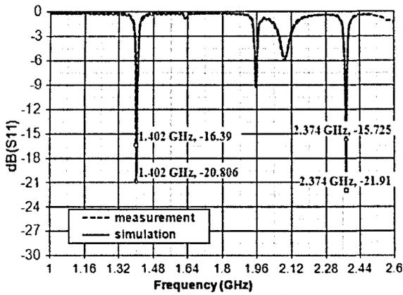
Figure 4: Simulation and Measurement of Return Loss  $S_{11}$
