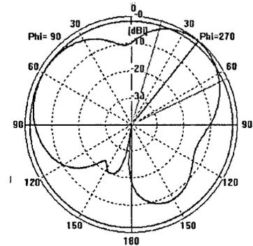
Figure 7: Radiation Pattern for 2.4GHz
