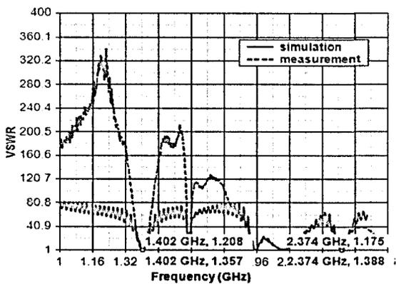
Figure 5: VSWR for simulation and measurement
