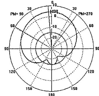
Figure 6: Radiation Pattern for 1.2GHz
