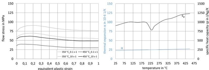
Figure 1: Determined thermomechanical (left) and thermodynamic (right; thermal expansion is from [14], specific heat capacity was measured) material behaviour of EN AW-6060
