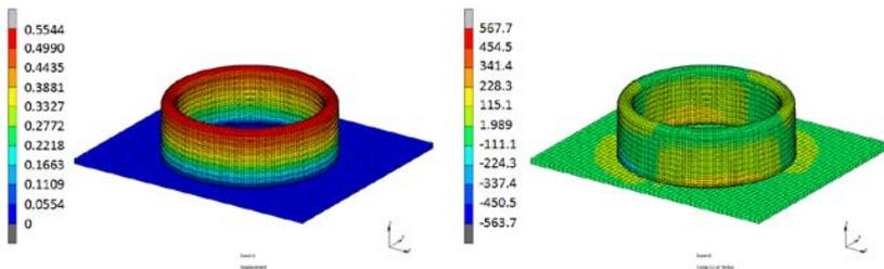
Figure 10. Simulated WAAM of magnesium cube up to room temperature (left: displacement; right: xy stresses)
