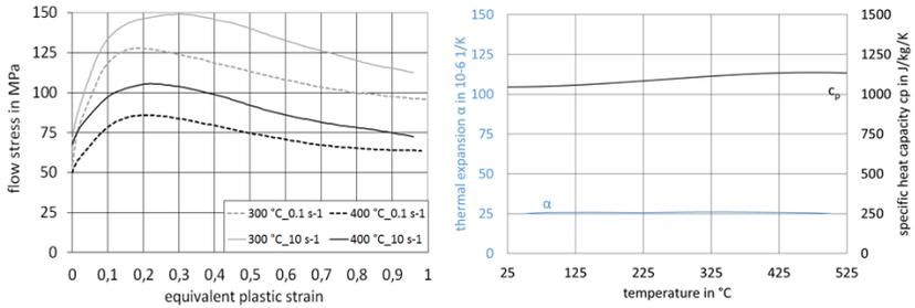
Figure 4. Determined thermo-mechanical (left) and thermo-dynamic (right) material behaviour of molten and solidified AZ31 wire
