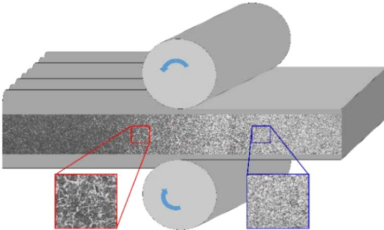
Figure 11. Change of microstructure in a hot rolled WAAM wall
