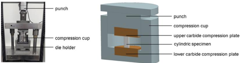
Figure 2. Setup for the compression tests (left: Galdabini Quasar 50 kN; right: compression cup for isothermal conditions)
