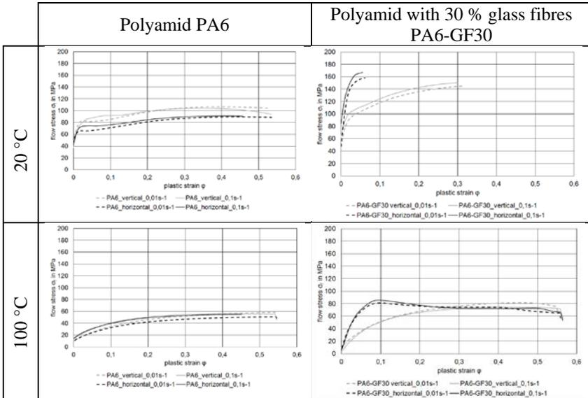
Figure 3. Comparison of the forming behaviour of polyamide with (right) and without glass fibres (left) at different temperatures (20 °C in the upper line; 100 °C in the lower line) and for varied strain rates (0.01 s<sup>-1</sup> and 0.1 s<sup>-1</sup>)
