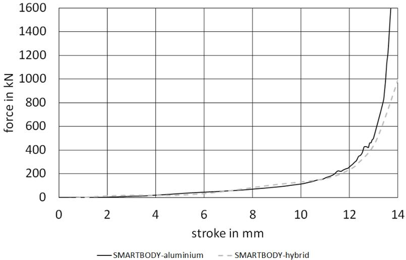
Figure 8. Comparison of the forging force for a monolithic aluminium alloy EN AW-6060 and a hybrid aluminium-plastic compound of EN AW-6060 and PA6
