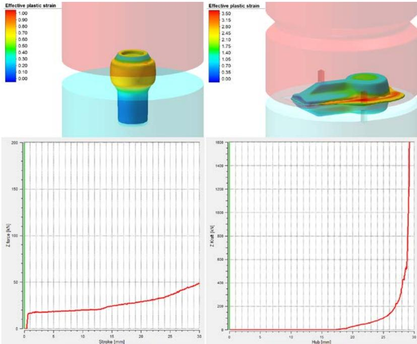
Figure 6. Simulated effective plastic strain and forces of forging the preform (left) and the final shape (right) at hydraulic press with 80 mm/s and initial temperature of 400 °C
