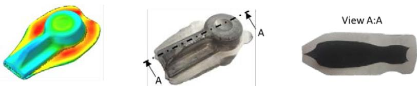
Figure 7. Forging of hybrid SMARTBODY (left: FEM; middle: real forging; right: cut over the length, black: polyamide; grey: aluminium)
