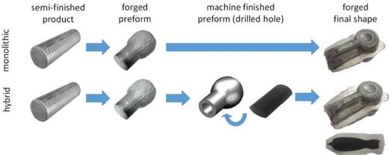
Figure 5. Investigated processes for monolithic and hybrid materials for the SMARTBODY
