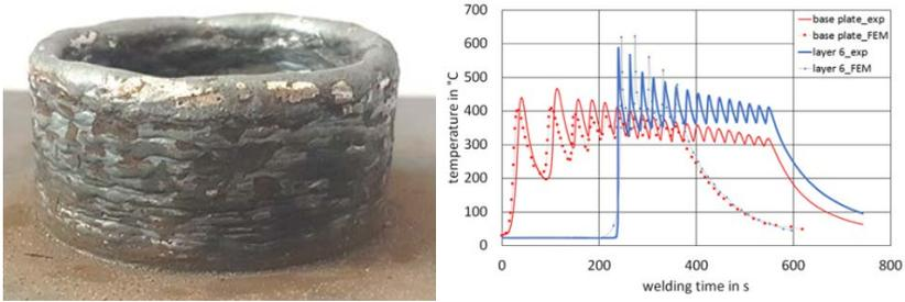
Figure 9. Magnesium WAAM tube (20 layers) and the comparison of measured and simulated temperature field
