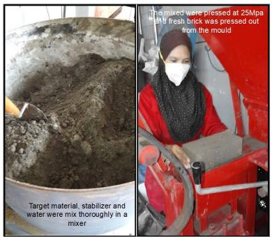
Figure 2. Fabrication of LSP Bricks Materials were throughly mixed and pressed.
