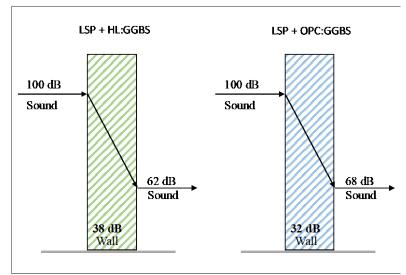
Figure 5: Schematic drawing of sound transmission loss of LSP Brick-wall
