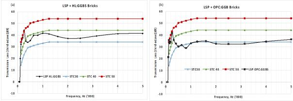
Figure 4: Transmission loss vs frequencies for LSP Brick stabilised with (a) HL:GGBS and (b) PC:GGBS
