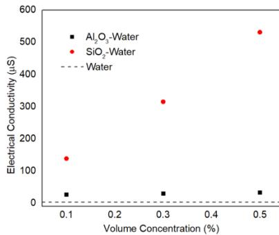
**Fig. 4.** Electrical conductivity against volume concentration of  $Al_2O_3$  and  $SiO_2$  with water as base fluid
