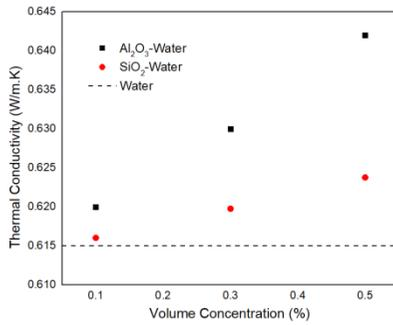
**Fig. 3.** Thermal conductivity against volume concentration of  $Al_2O_3$  and  $SiO_2$  with water as base fluid
