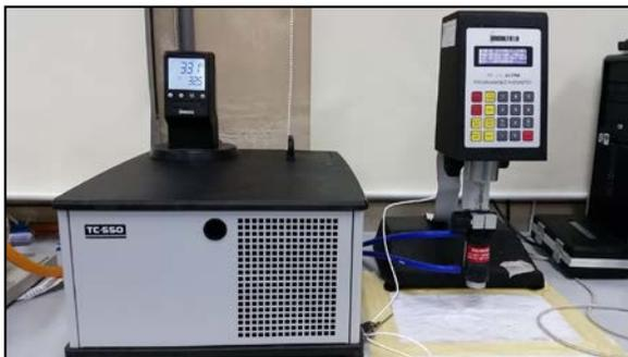
(c) Low Viscosity Digital Viscometer (LVDV-III) Ultra Programmable Rheometer
