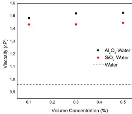
**Fig. 5.** Viscosity against volume concentration of Al<sub>2</sub>O<sub>3</sub> and SiO<sub>2</sub> with water as base fluid
