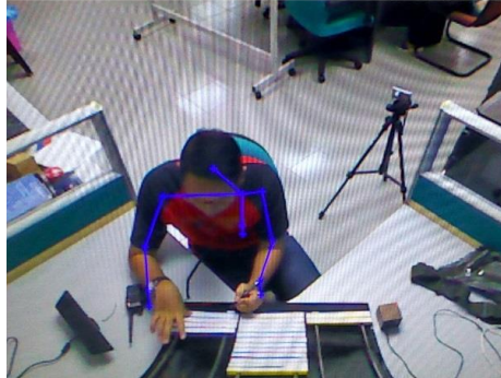
Figure 2: Upper Body Movement Tracking by Kinect®
