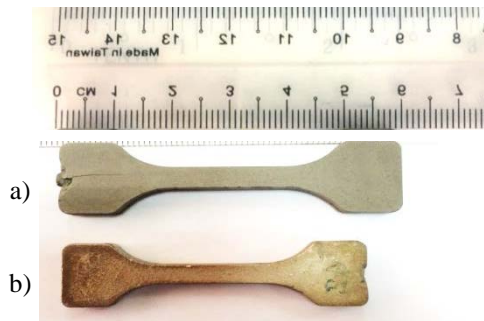
Figure 5: Dimensional comparison between a) green injection moulded part and b) sintered part
