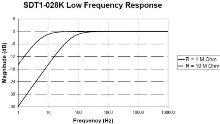
Figure 3: Low-frequency response of the piezo-film sensor.
