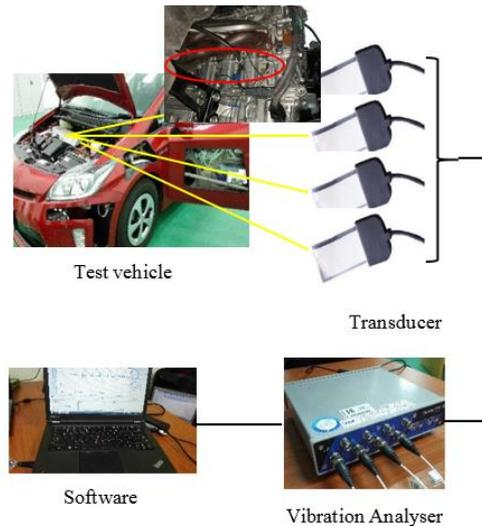
Figure 2: HEV engine signal acquisition process flow diagram.
