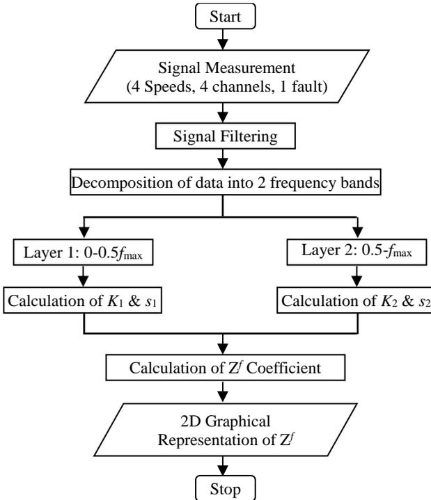
Figure 1: Hybrid vehicle engine monitoring flowchart using Z-freq.
