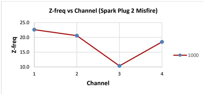
Figure 8: Z-freq plot for channel 3 misfire.
