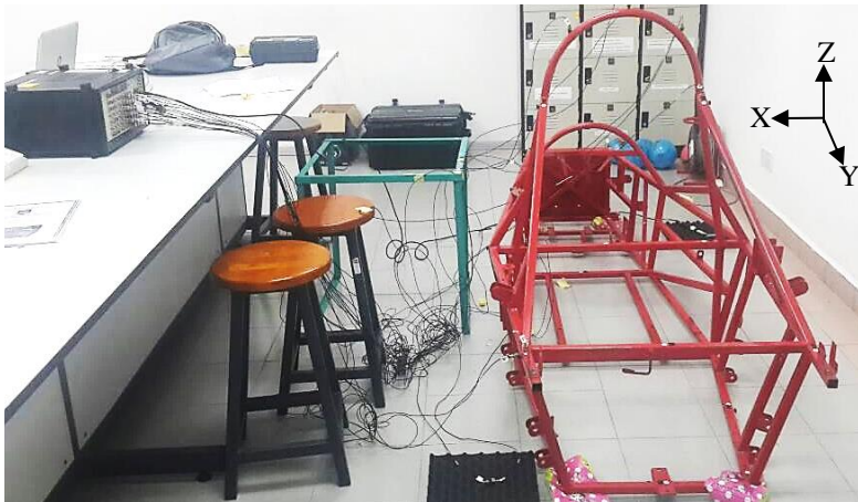
Figure 4: Experimental Modal Analysis and Operational Modal Analysis experimental set-up.
