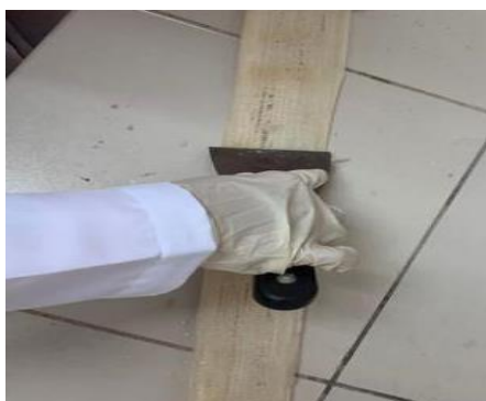
Figure 1. Scraping process of banana pseudo-stem fibres
