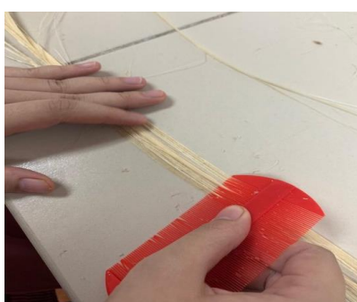
Figure 2. The combing process of banana pseudo-stem fibre
