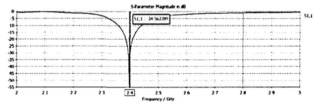
Figure 9: Antenna return loss
