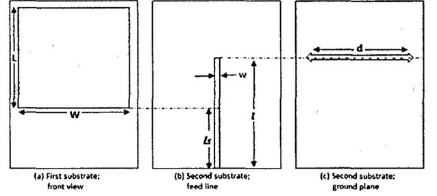
Figure 3: Antenna geometry.
