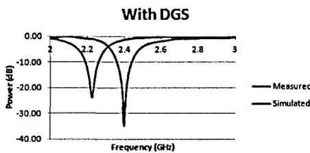
Figure 14: Return loss for antenna with DGS
