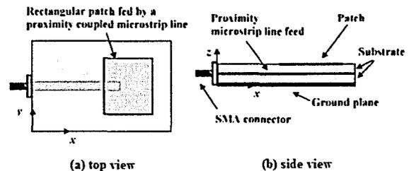
Figure 1: The geometry of proximity coupler feed antenna [6].
