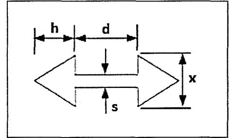
Figure 4: Geometry of shapes of DGS slot.
