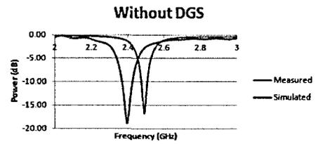
Figure 15: Return loss for antenna without DGS
