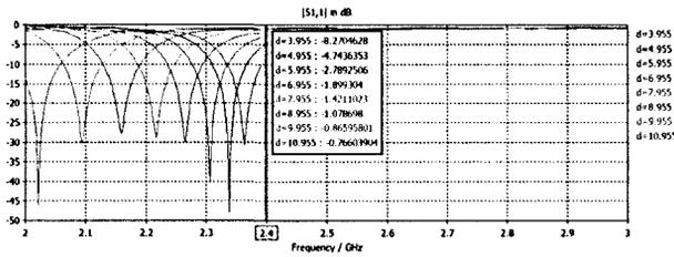
Figure 12: Return loss by varying DGS length,  $d$ .
