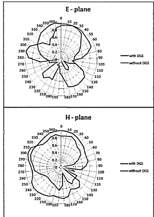
Figure 16: Antenna radiation pattern.
