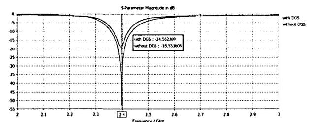
Figure 11: Simulated return loss
