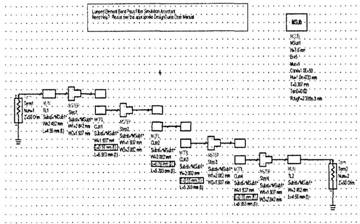
Figure 4. Ideal parallel coupled bandpass filter.
