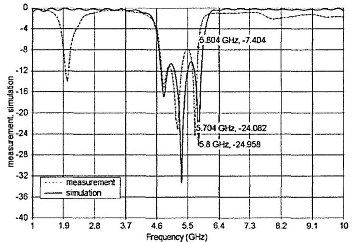
Figure 7. Simulated and measured of return loss, S11.
