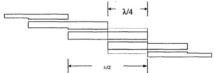
Figure 3. Third order edge-coupled  $\lambda/2$  pass filter-notice that the coupling resonators are  $\lambda/4$  long (depicted by gray area).
