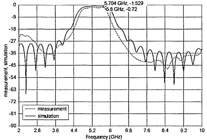
Figure 6. Simulated and measured of insertion loss, S21.
