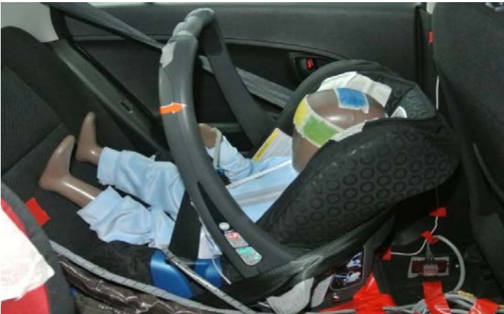
Figure 8: P1.5 dummy installed inside the tested vehicle using a three-point belt
