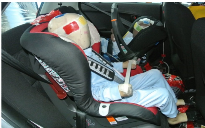
Figure 6: P3 dummy installed using three-point seatbelt
