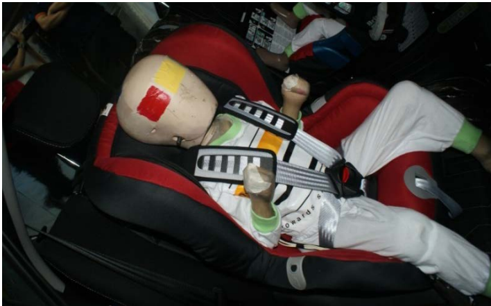
Figure 5: P3 dummy installed inside the car using ISOFIX and top tether
