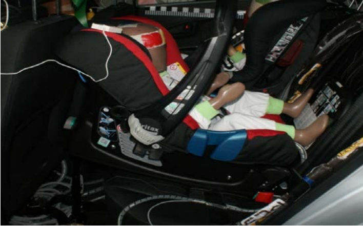
Figure 7: P1.5 dummy placed inside vehicle using ISOFIX with base support
