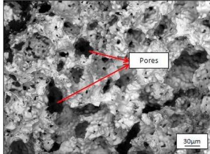
Figure 7: The porosity that affects the mechanical strength of the sintered specimen.
