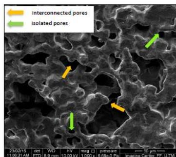
Figure 6: The example of interconnected pores and isolated pores in the as-sintered specimen.
