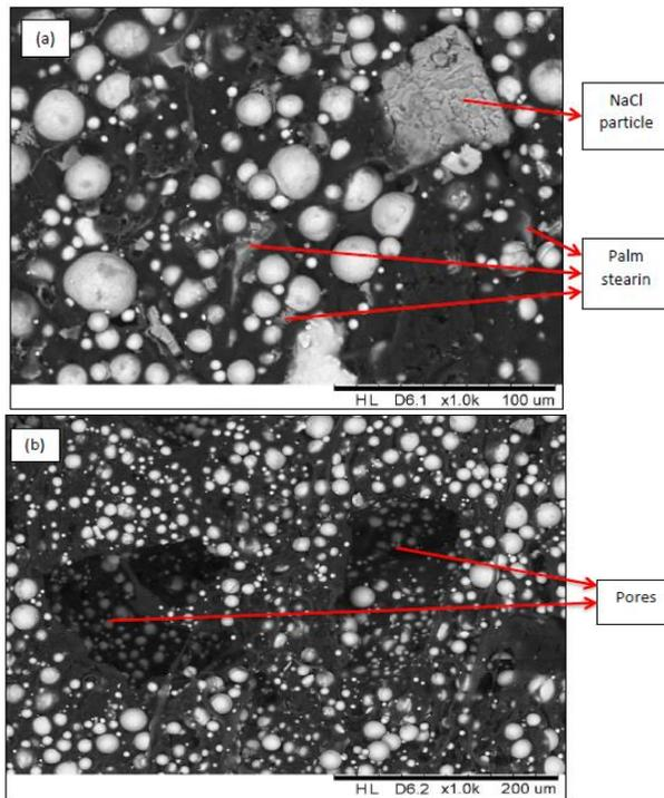
Figure 4: Solvent debinding and water leaching process, a) before and b) after.
