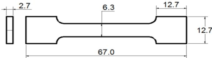
Figure 2: Tensile bar sample
