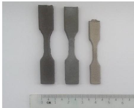
Figure 5: Shrinkage effect before and after sintering (a) green part (b) PS and NaCl debound part (c) as-sintered part
