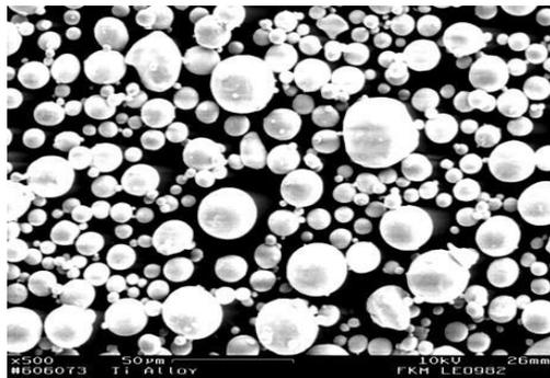
Figure 1: SEM particle of Ti-6Al-4V
