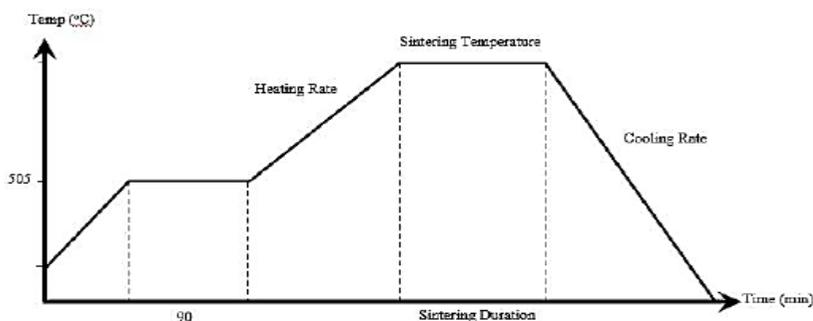
Figure 3: Pyrolysis graph and heating cycle sintering process
