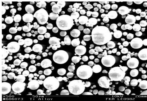
Figure 1: SEM particle of Ti-6Al-4V
