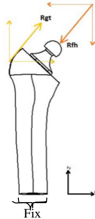
Fig. 6. Loading and boundary setup condition
