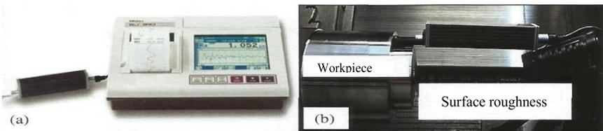
Figure 17: (a) Mitutoyo SurfTest SJ-310 portable surface roughness tester (b) Placement of surface roughness tester on the workpiece surface
