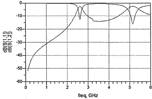
Figure 12: DBSRR circuit with **SIX** meanders microstrip simulation.
