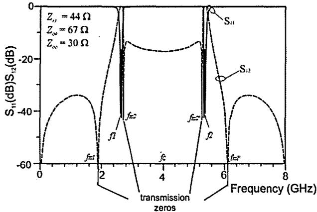
Figure 2: Ideal circuit microstrip simulation result
