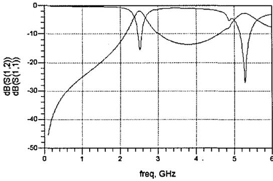
Figure 8: DBSRR circuit with **THREE** meanders microstrip simulation.
