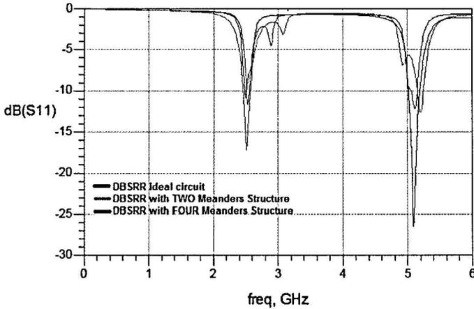
Figure 13: Comparison microstrip simulation results for ideal DBSRR, DBSRR circuit with **TWO** and **FOUR** meanders structure (S11).
