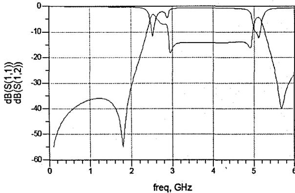
Figure 10: DBSRR circuit with **FOUR** meanders microstrip simulation.
