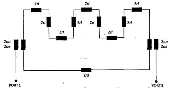
Figure 5: DBSRR circuit with **TWO** meanders structure.
