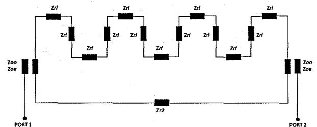
Figure 7: DBSRR circuit with **THREE** meanders structure.
