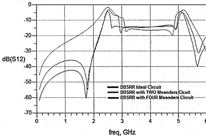
Figure 14: Comparison microstrip simulation results for ideal DBSRR, DBSRR circuit with **TWO** and **FOUR** meanders structure (S12).
