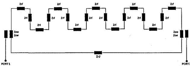
Figure 9: DBSRR circuit with **FOUR** meanders structure.
