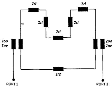
Figure 3: DBSRR circuit with **ONE** meander structure.
