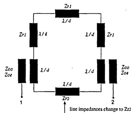
Figure 1: Circuit diagram of DBSRR topology.
