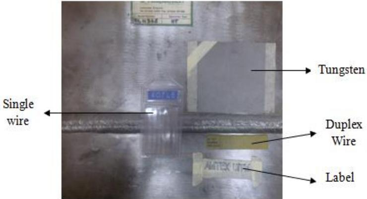
Figure 7: Arrangement on the Flawed Specimen.
