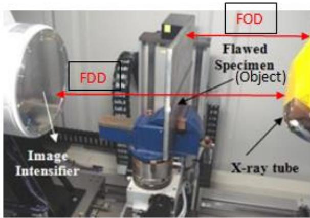
Figure 5: Radiography Source, Detector and Flawed Specimen Arrangement.
