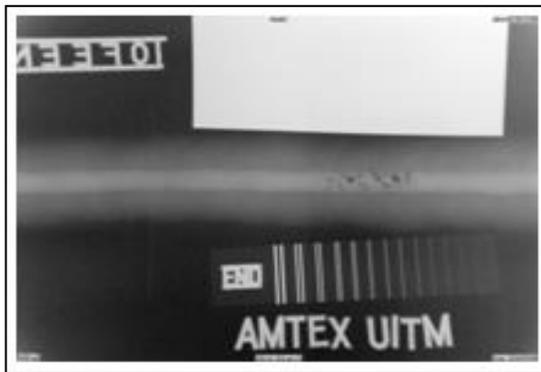
Figure 8: Radiographic Image of the Flawed Specimen.
