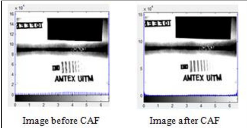
Figure 9: Image and Its Histogram Using Circular Average Filter (CAF).
