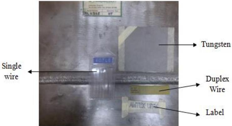
Figure 7: Arrangement on the Flawed Specimen.
