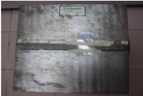
Figure 6: Sample of Welded Flawed Specimen.
