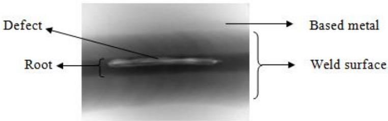
Figure 1: Flawed Specimen Distribution.
