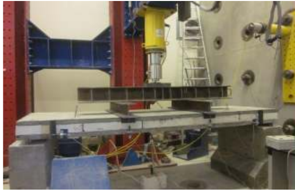
Figure 6: RC sandwich panel with AAC infill during a 4-point load bending test.
