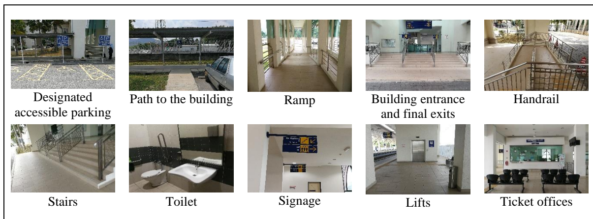
Figure 1 Types of facilities for PWDs to be provided at ETS railway station
