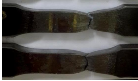
Figure 10: Untreated Specimen –break in weld metal and HAZ
