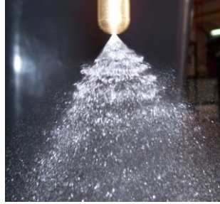
Figure 1: Typical spray pattern for hollow cone atomizer.
